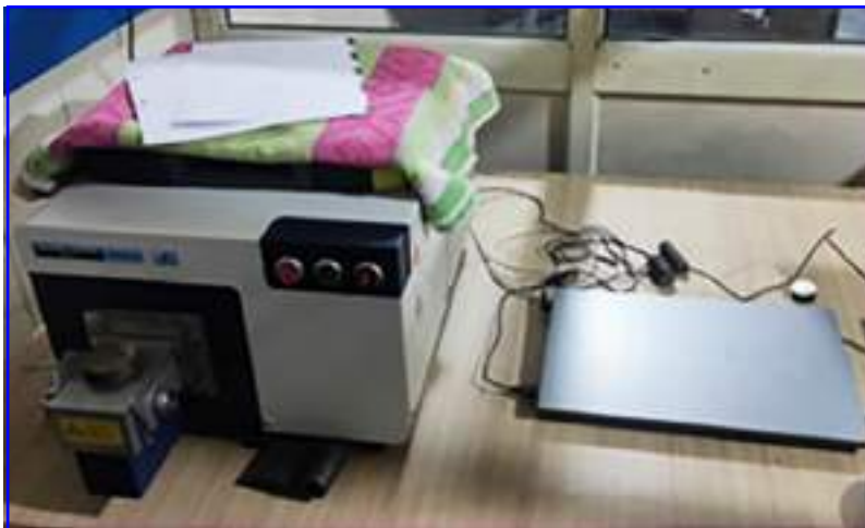
2. In-house spectrometer to verify the composition mentioned in test certificate
